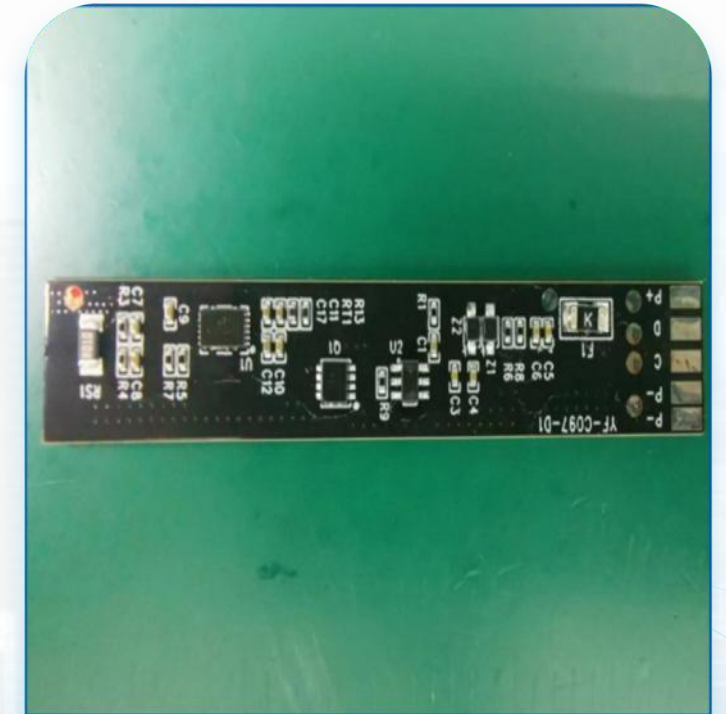
Security monitoring battery protection panel
